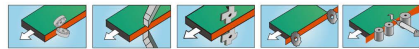
1. 拼光 Butting 2. 刮边 Scraping 3. 精修 Fine trim 4. 前后齐头 End Cuffing 5. 涂胶贴边 Gluing
