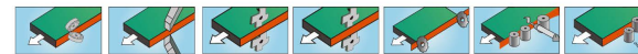
1. 拼光 Butting 2. 刮边 Scraping 3. 精修 Fine trim 4. 粗修 Rough trim 5. 前后齐头 End Cuffing 6. 涂胶贴边 Gluing 7. 预铣 Pre-milling
