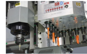
自动换刀主轴+9L钻组 Automatic tool changer spindle +9L boring head
