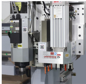
自动换刀主轴+9L钻组 Automatic tool changer spindle +9L boring head
